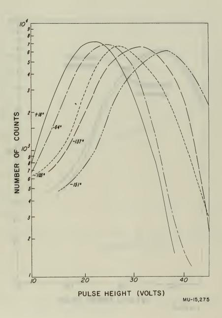
Fig. 7. Pulse height spectra for decreasing temperature in argon at 75 psi. Cm<sup>244</sup> source.
